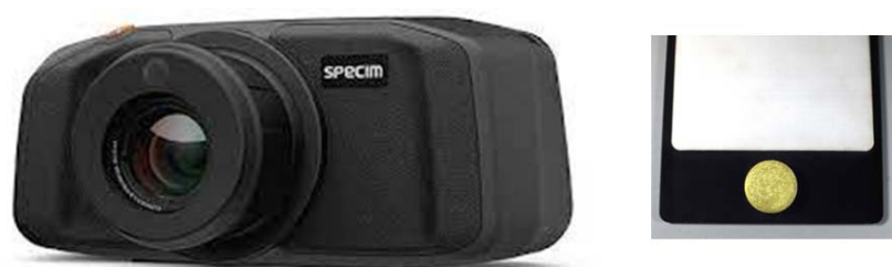
Fig. 1. Specim IQ camera (on the left) and the way of placing an example tablet on a reference plate (on the right).
